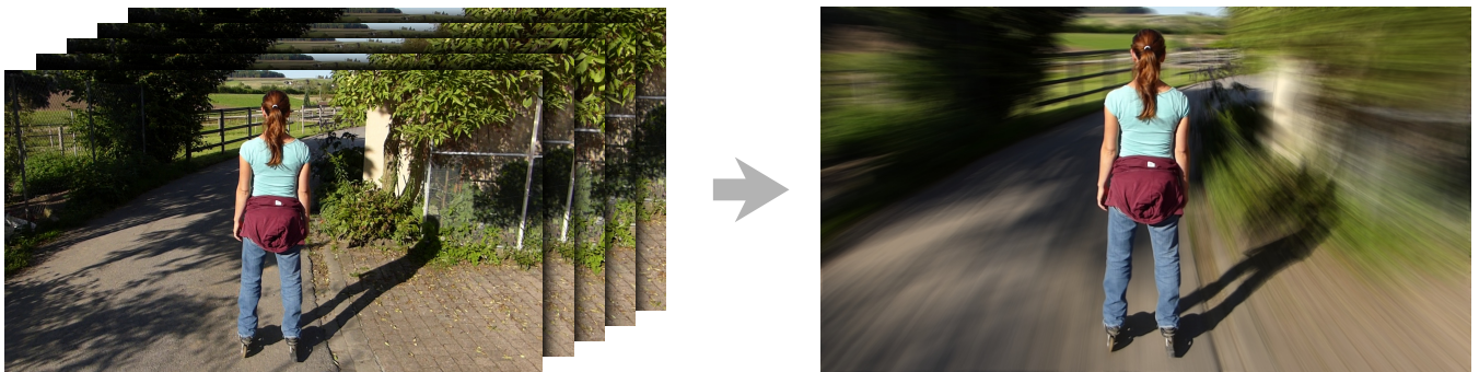
Figure 1: From a hand-held video (left) 22 frames are selected, stabilized on the main subject, temporally interpolated and averaged to create a single image (right) that conveys a sense of motion, simulating a single stabilized long time exposure photo.
