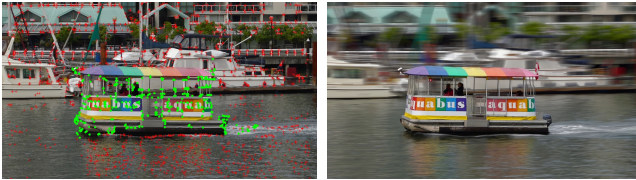
Figure 3: Left: One of the source frames with tracked features. The automatically selected features (green) include some outliers. They are used for a robust rigid alignment of each frame before final averaging. Right: Fully automatic result with our pipeline.
